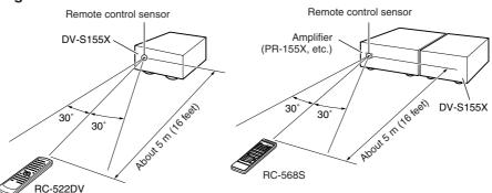
Point the remote controller toward the remote control sensor.
